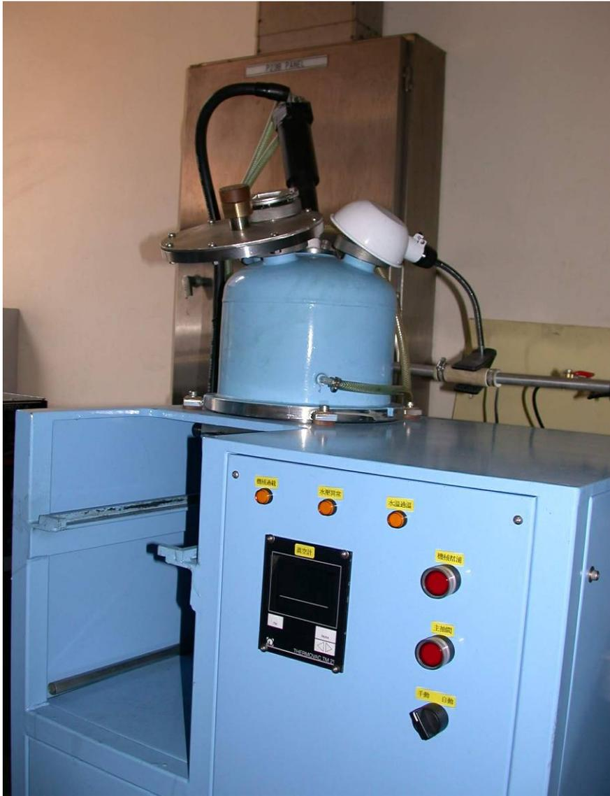
Figure 3.2 Photograph of the arc melting device.
