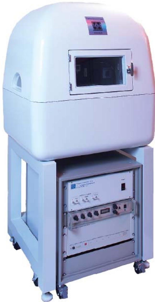
Figure 3.14 The picture of Hysitron Triboindenter system.
